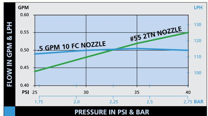
Flow control nozzles (10FC) are an excellent low cost option when system pressure ranges between 25-50 PSI (1.7-3.4 BAR). When system pressure differences are more extreme the Nelson Mini Regulator or Mini Regulator Drain Check are ideal products.
