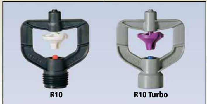
A special motor (brake) design in the R10 Turbo Rotators has more resistance to maximize radius, reliability, and uniformity.
