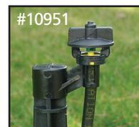
The deflector cap is used to reduce the R5 Rotator radius down to 3-4 feet (0.9-1.2 m) for watering newly planted trees.
